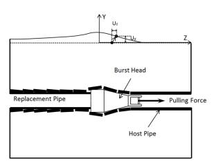
Schematic of the pipe bursting process
