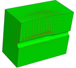
Calculated ground motion caused by the burst head
