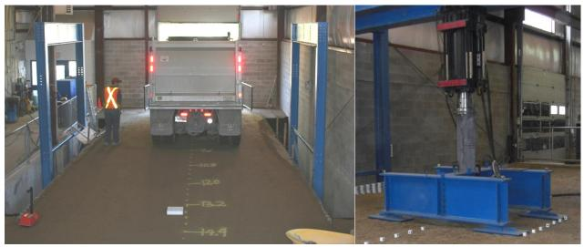
Use of the GeoEngineering Laboratory to conduct full scale testing of a large span metal culvert under both real and simulated truck loading.
