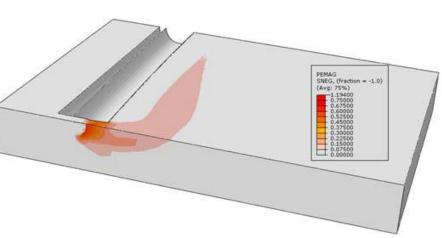
Mohamed inspects a test pipe. Contours of plastic soil strain below and ahead of the test pipe.
